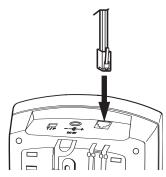
3. Insert the supplied AC adapter's barrel plug into the DC 12V jack on the back of the base.
